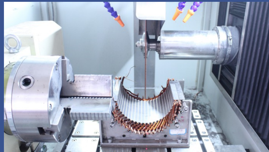
Customizable R-axis And cutting fixture tooling
